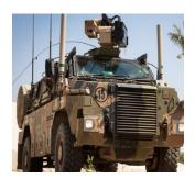
"Purpose designed and built to exacting A.D.F. [Australian Defence Force] requirement specifications for use on Bushmaster vehicles [illustrated left] accessing the USA / Australian W.G.S. [wideband global SATCOM] Geo-stationary satellite constellation. EM Solutions' SOTM terminal aims to provide a very high availability connection with the satellite even while traveling at 100km/hour on the highway or 40km/hour off-road.
